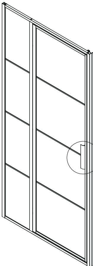
Install handle at the door. Lock with M4\*18 screws ( totally 2 screws)
